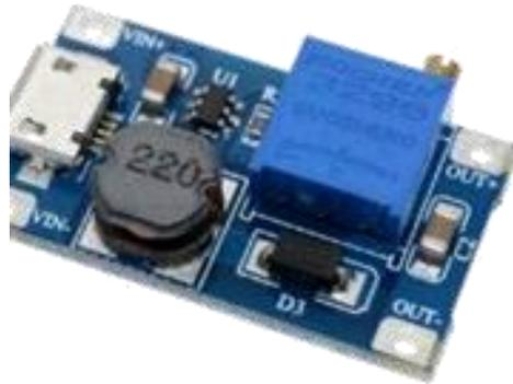
Gambar 4. Modul *Step Up Booster* MT 3608
