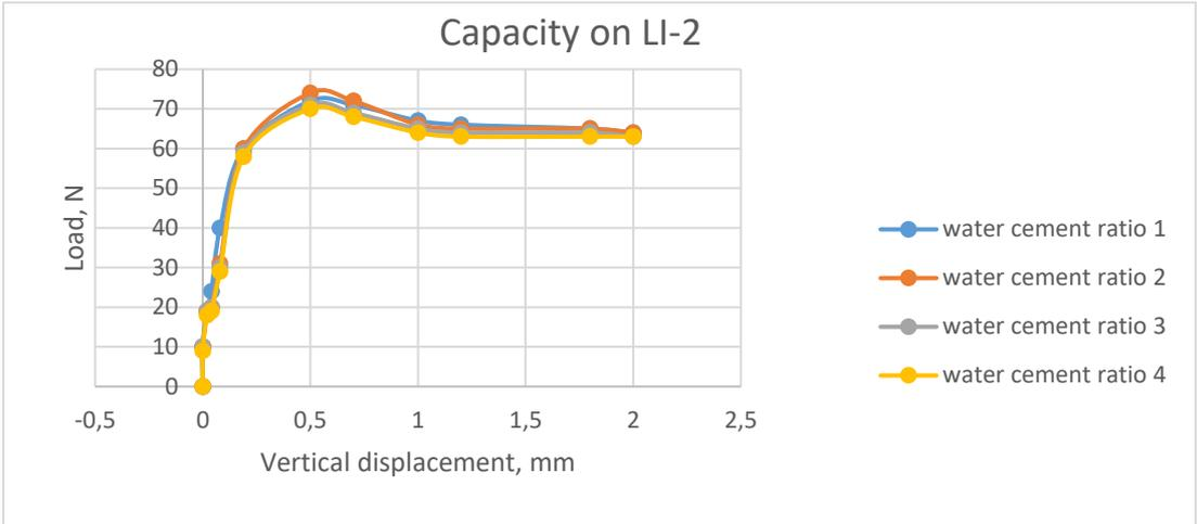
Figure 7. L-S Curve of PLT on LI-2 at Various w/c Ratio at 3 Days Curing
