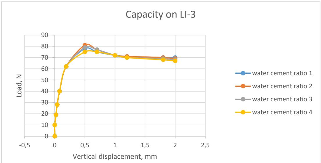
Figure 8. L-S Curve of PLT on LI-3 at Various w/c Ratio at 3 Days Curing
