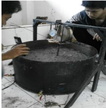
Figure 2. Pile loading test was being carried out
