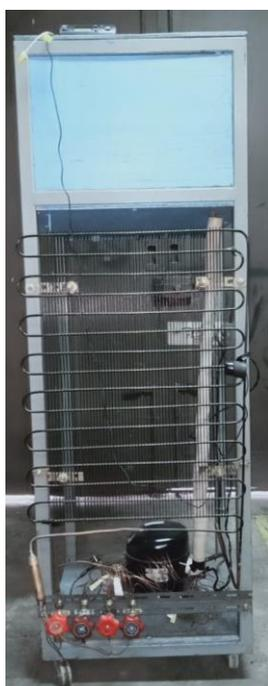
Gambar 1. Alat Peraga Praktik Mesin Pendingin Refrigerator
