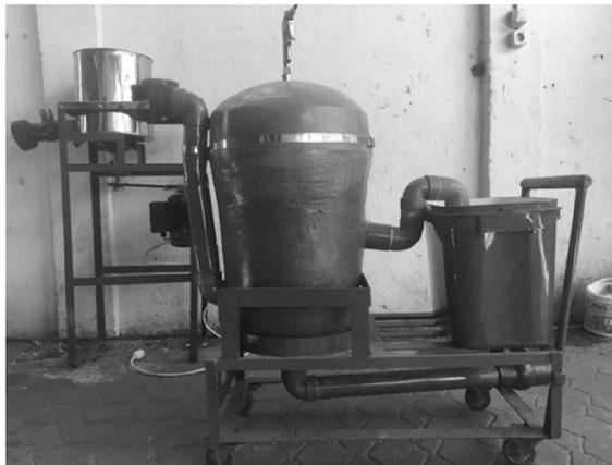
Gambar 1. Reaktor Gas Tipe *Fixed Dome* Multi Input.
