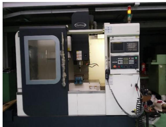
Gambar 2. Mesin CNC milling Hartford Pro 800 3-Sumbu (Hartford, 2018)
