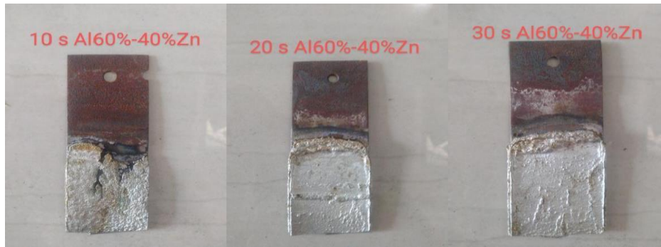
Figure 4. The Results of The Galvalume Process With a Composition of 60 % Aluminium and 40% Zinc, With a Hot Dip Time of 10 Seconds, 20 Seconds, and 30 Seconds.
