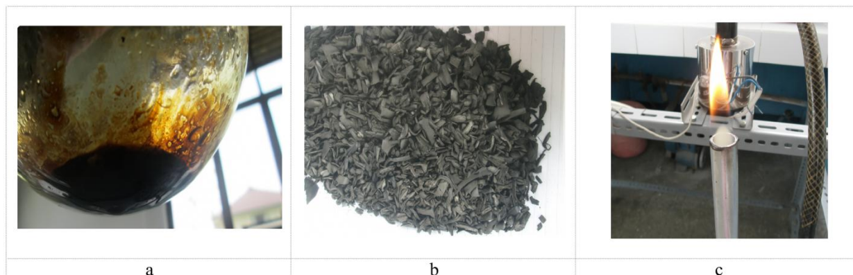
Figure 4. Products of Pyrolysis: (a) Bio-Oil, (b) Charcoal, and (c) Combustible Gas.
