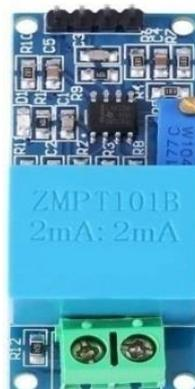
Gambar 4. Modul Sensor Tegangan ZMPT101B
