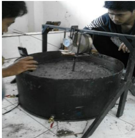
Figure 2. Pile loading test was being carried out
