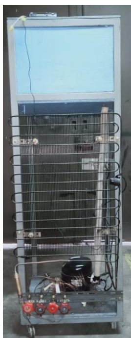
Gambar 1. Alat Peraga Praktik Mesin Pendingin Refrigerator
