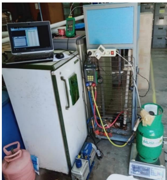
Gambar 3. Set Up Alat Pengujian Mesin Pendingin Refrigerator
