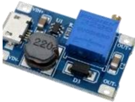
Gambar 4. Modul Step Up Booster MT 3608
