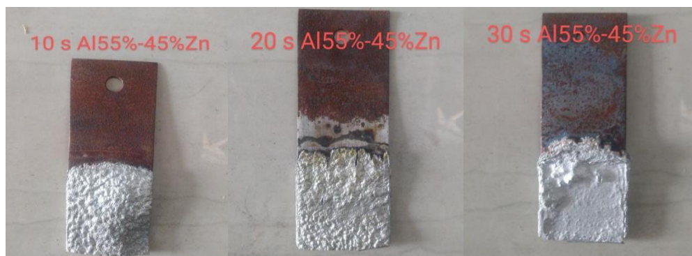
Figure 3. The Results of The Galvalume Process with a Composition of 55% Aluminium and 45% Zinc, with a Hot Dip Time of 10 Seconds, 20 Seconds, and 30 Seconds.
